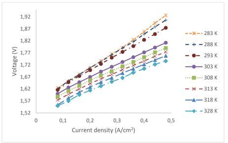
*Figure 1* Polarisation curve at different temperatures.
