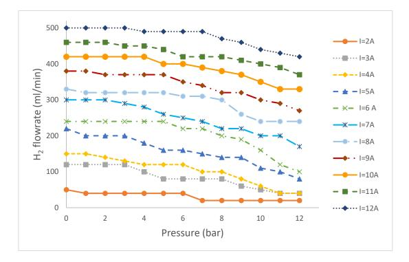
**Figure 12** Hydrogen production as a function of the pressure for different intensities. In order to compare the production drop between the productions at different intensities, the production drop percentage was calculated as shown in equation 4.
