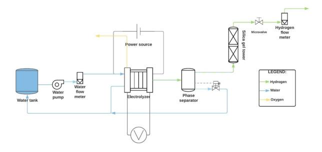
Figure 7 Conceptual scheme of the electrolysis equipment.
