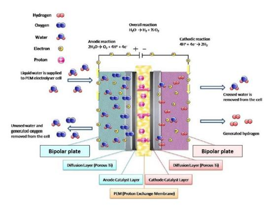
Figure 5 Working principles and schematic of a PEM electrolyzer.
