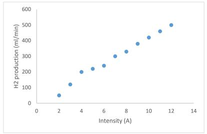
*Figure 8* Hydrogen production as a function of intensity.
