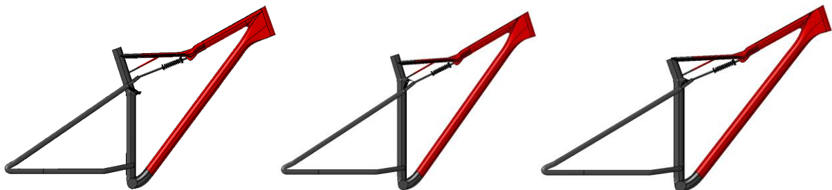
Figure 58: Best, less stressed and lightest S-Works Epic geometry, respectively.
