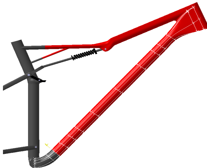
Figure 28: Diagonal tube geometry sketch.
