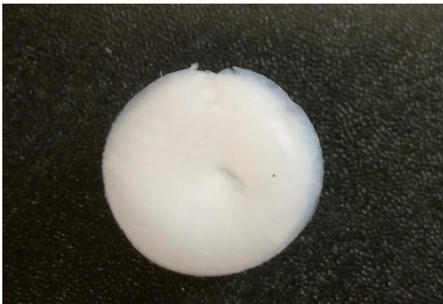
**Figure 17.** Top-view of an aerogel
