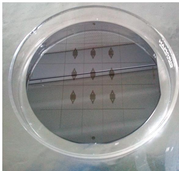
Figure 9: Silicone wafer used to microfabricate the microfluidic chips. The design is repeated 9 times to obtain a large number of chips in the process.
