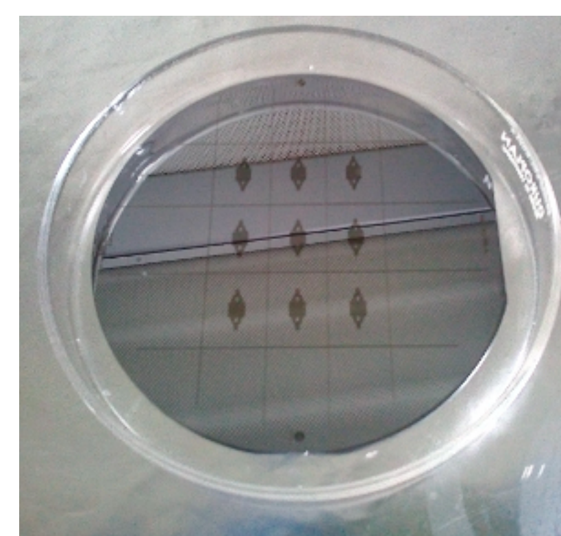
Fig. 3. Redesign of microfluidic chip design with scale [5] Fig 4. Wafer used in microfabrication to make the chips
