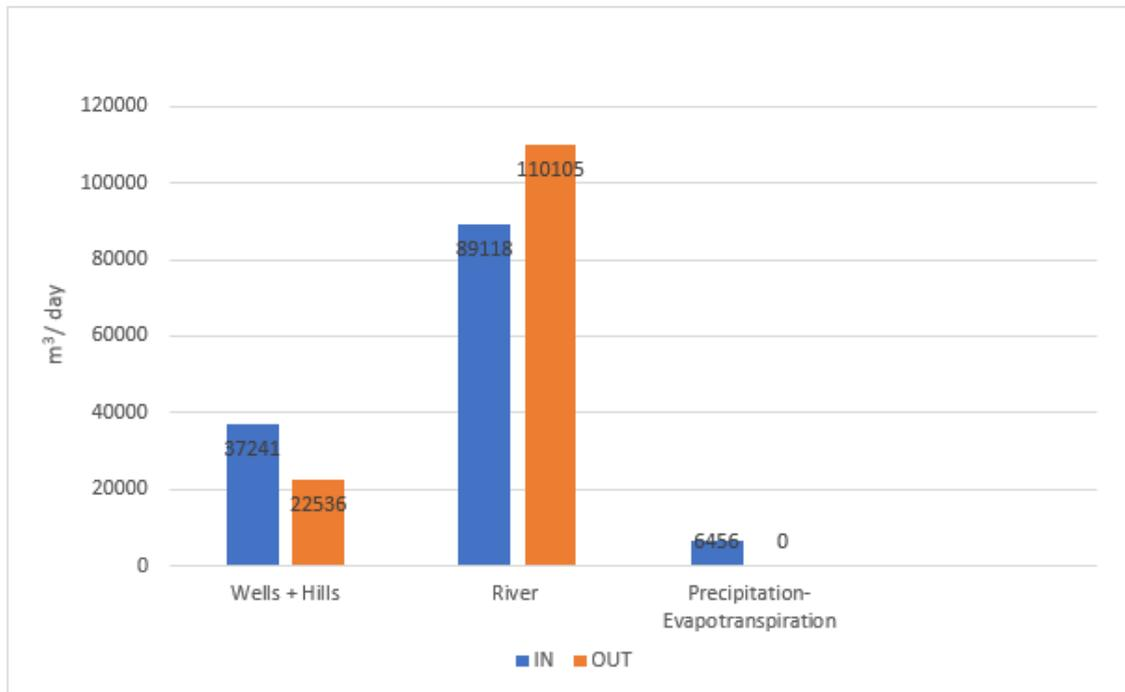
Diagram 3. Volumetric flow comparison for the scenario 3
