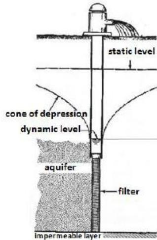
Figure 11: The relationship between the pumping well and the aquifer. [4]
