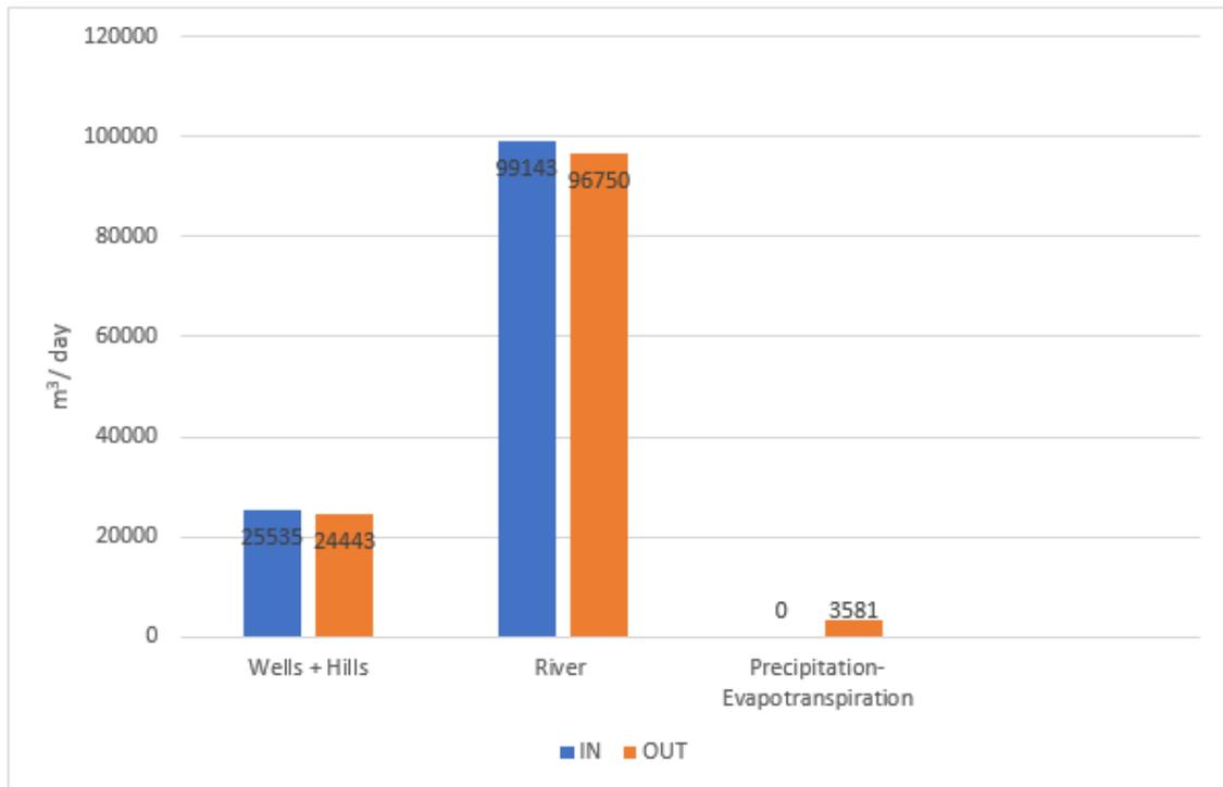
Diagram 5. Volumetric flow comparison for the scenario 5
