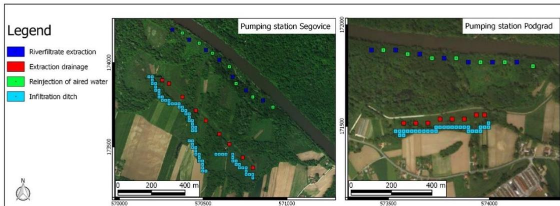
Figure 18. Pumping station Segovci and Podgrad
