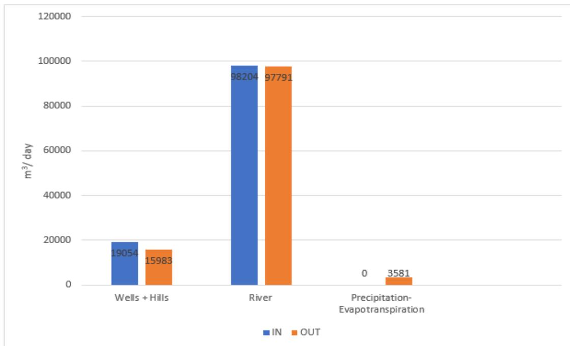
Diagram 6. Volumetric flow comparison for the scenario 6
