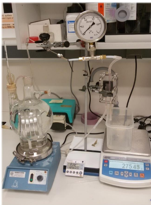
Figure 6. 2. Homemade cross-flow filtration system
