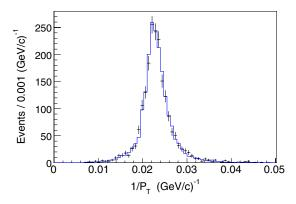
FIG. 4 (color online). Distribution of  $C^+$  for same-side (SS) pairs in the central  $\eta$  region of (-0.3,0). The crosses are the data, and the solid histogram is the generator-level distribution normalized to the data.
