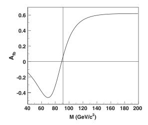
FIG. 3. Typical dependence of  $A_{\rm fb}$  as a function of the lepton-pair invariant mass. The curve is an analytic calculation. The vertical line is at  $M=M_Z$ .
