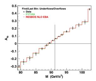
FIG. 15 (color online). Fully corrected  $A_{\rm fb}$ . The measurement uncertainties are uncorrelated bin-by-bin unfolding estimates. The vertical line is  $M=M_Z$ . The PYTHIA calculation uses  $\sin^2\theta_{\rm eff}^{\rm lept}=0.232$ . The EBA-based RESBOS calculation uses  $\sin^2\theta_W=0.2233$  ( $\sin^2\theta_{\rm eff}^{\rm lept}=0.2315$ ).
