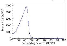
FIG. 9 (color online). Calibrated  $P_{\rm T}$  distribution for the muon with the smaller  $P_{\rm T}$ . The crosses are the background-subtracted data and the solid histogram is from the simulation.
