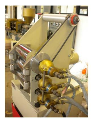
The Univex can take off, cool, and wind up flat films up to a max. film speed of 30 m/min.
