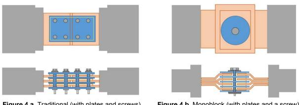
Figure 4.a. Traditional (with plates and screws)
