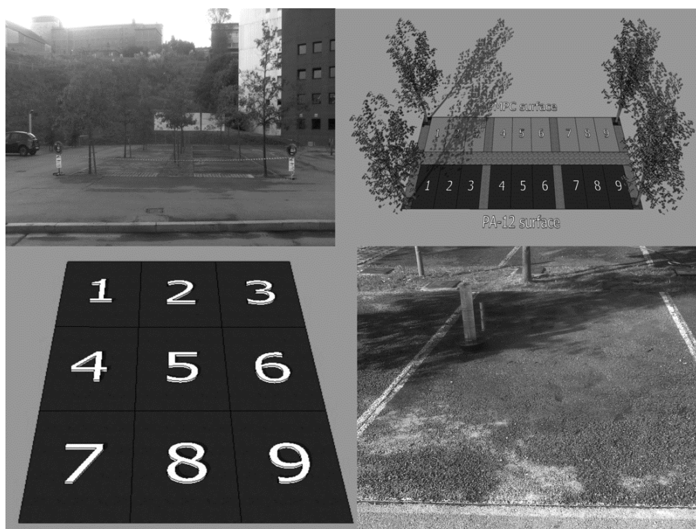
Figure 8. (Above) Scheme of the eighteen car parking bays analyzed, and (below) measurement zones selected within each car park bay and LCS on-site.
