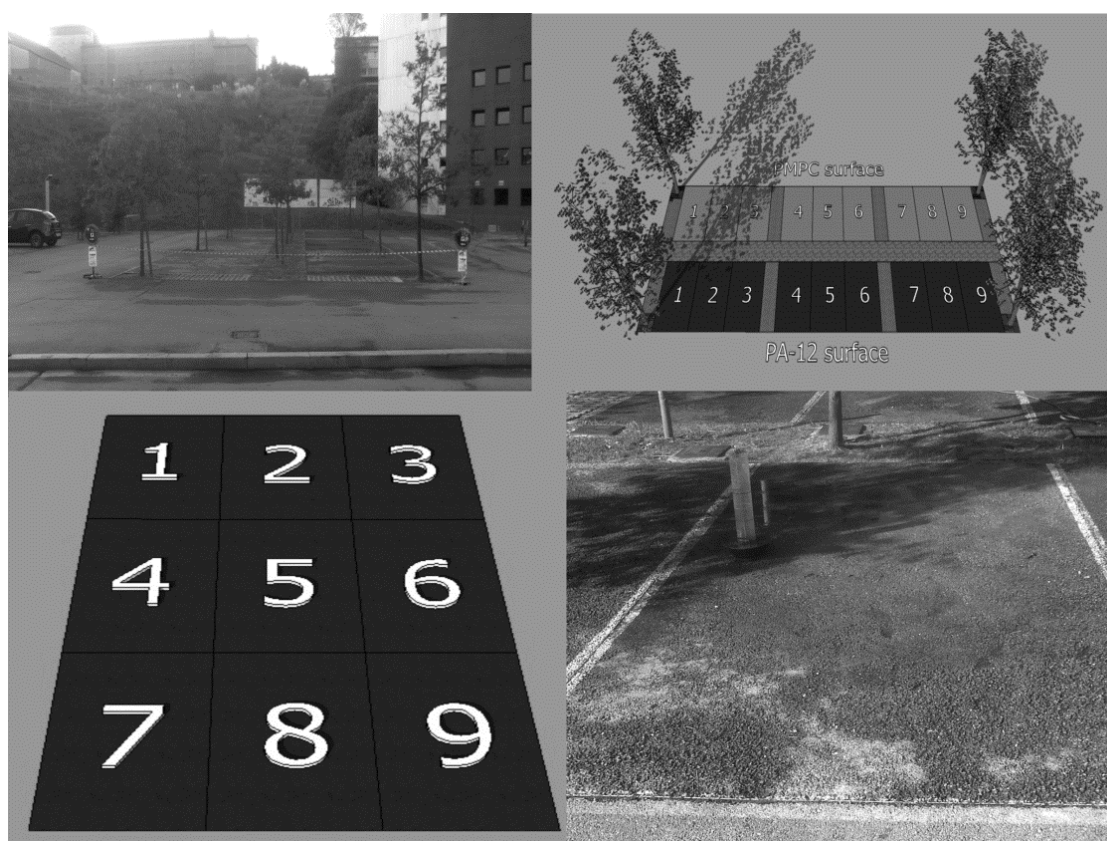
Figure 1. (Above) Scheme of the eighteen car parking bays analyzed, and (Below) measurement zones selected within each car park bay and LCS on-site.
