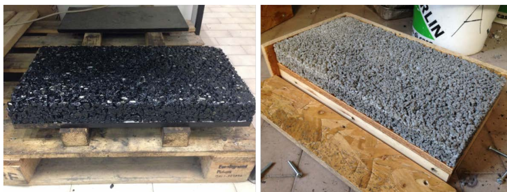
Figure 4. Porous surface materials: a) Porous asphalt (PA) and b) Porous Concrete (PC)
