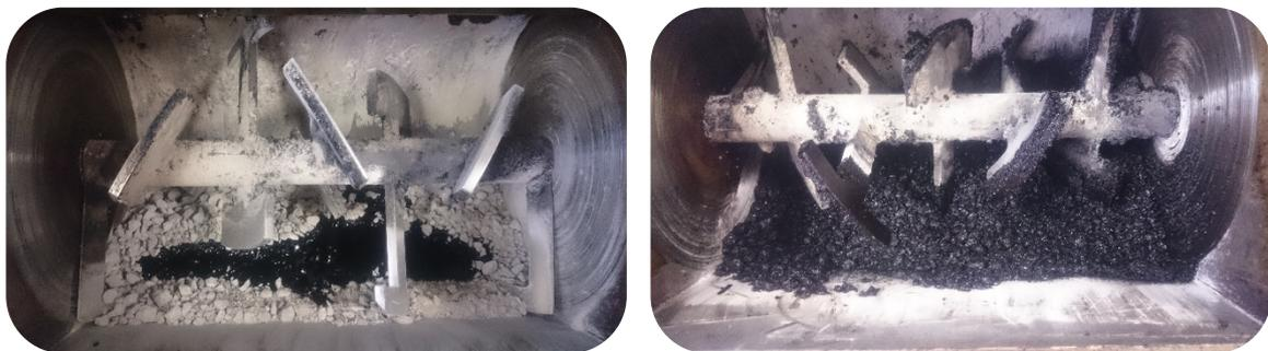
Figure 15. Addition of bitumen and final mixture
