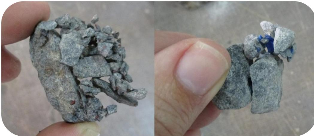
Figure 27. Aggregates with PE and PP
