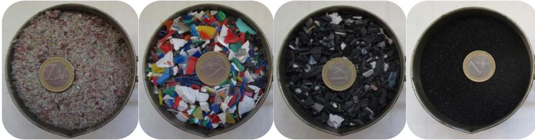
Figure 9. Selected polymeric waste: PE, PP, PS and ELT from left to right
