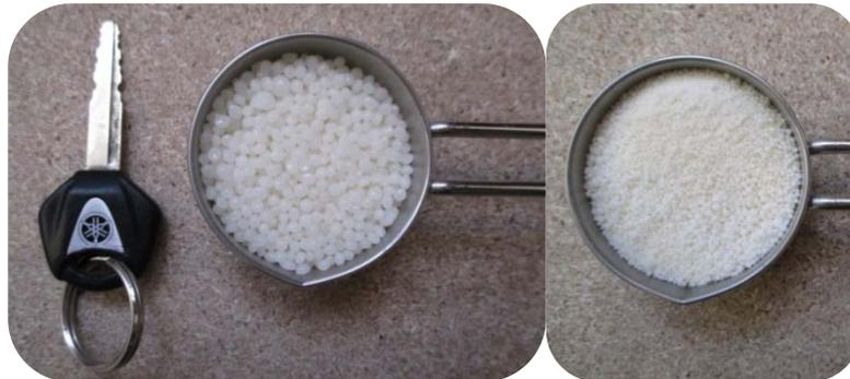
Figure 12. Additives: Left: Fischer – Tropsch wax. Right: Fatty acid amide wax
