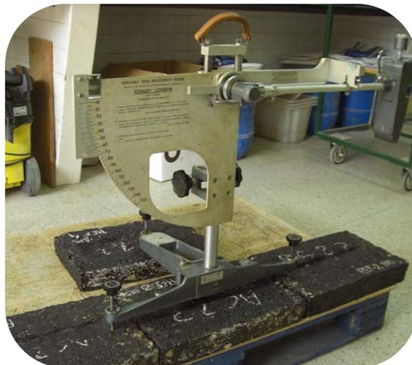
Figure 33. Evaluation of skid resistance
