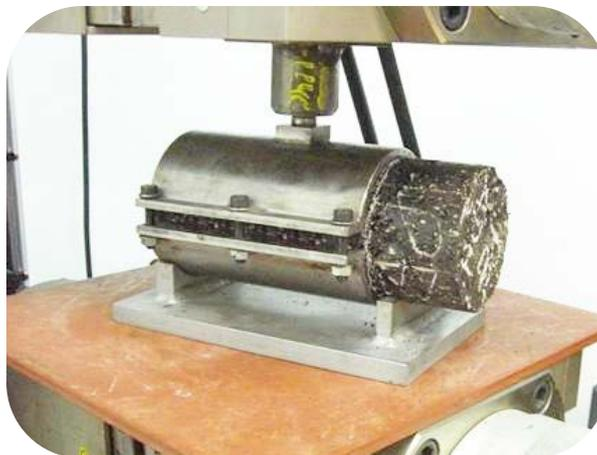
Figure 35. Test of static adherence between layers
