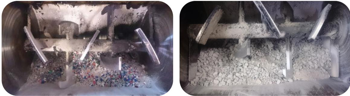
Figure 14. Polymeric waste poured on the aggregates and mixture without bitumen
