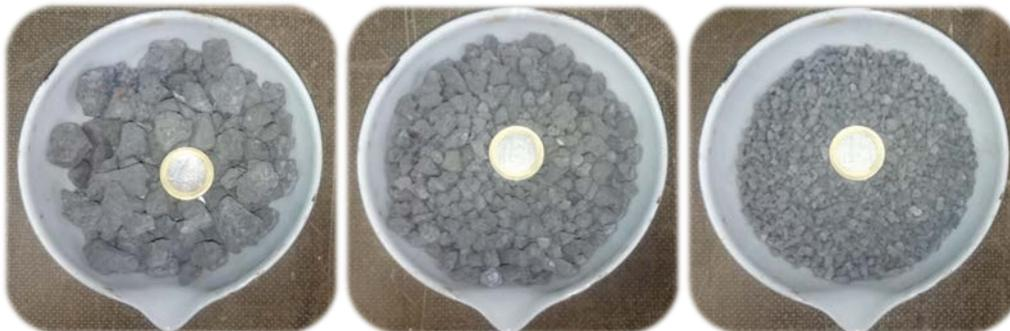
Figure 6. Black slag divided in three sizes. From left to right: 16/8, 8/4 and 4/2
