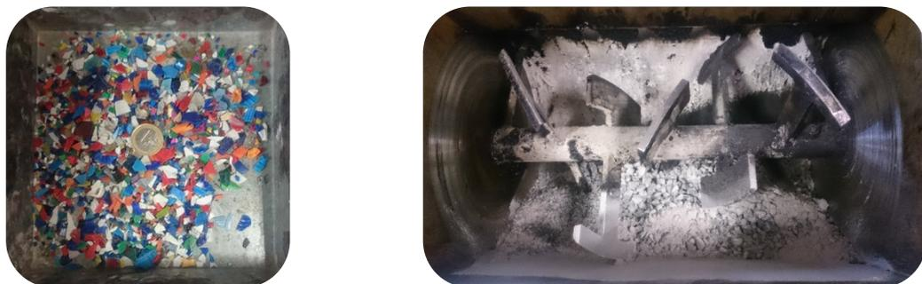
Figure 13. Polymeric waste (PP) and natural aggregate in the mixer
