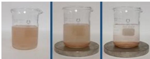
**Fig. 3.8. Separation process of the Fe<sub>3</sub>O<sub>4</sub>@SiO<sub>2</sub>@TiO<sub>2</sub>-WO<sub>3</sub> photocatalyst after the photocatalytic treatment of BPA in UP water in photoreactor 1 (Xe lamp).**
