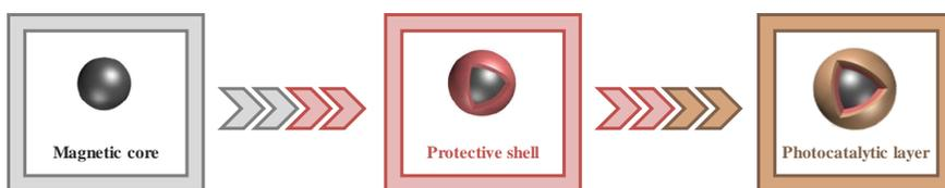
**Fig. 1.7. General structure of magnetic photocatalysts.**
