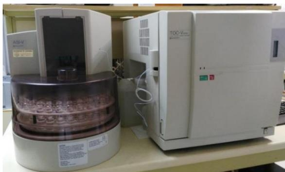
**Fig. 2.9. TOC-VCPH analyzer with auto-sampler ASI-V.**
