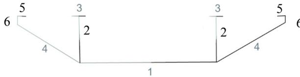
Fig. 3. Identification of the different plates composing the bridge deck.
