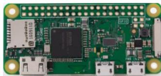
Figura 2.6: Raspberry Pi Zero W [26]
