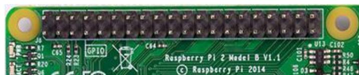
Figura 4.1: GPIO Raspberry Pi 2 B [23]
