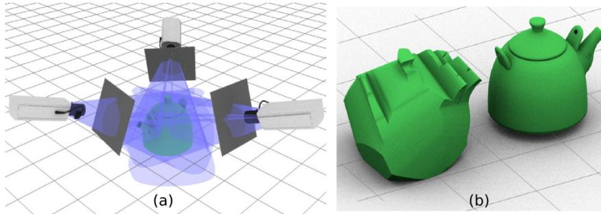
FIGURE 3.18: (a) Reconstruction scan seen from three different points of view. (b) The visual Hull of a teapot computed from three points of view (left) and the object (right).
