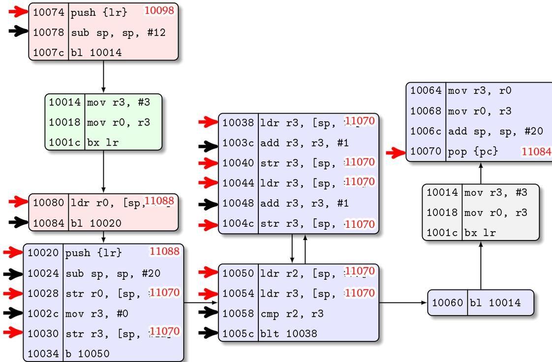
FIGURE 2.10: First phase of the *analysis*. Coarse slicing and *sp* computation.
