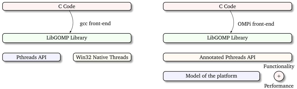
FIGURE 3.9: APIs involved in OpenMP parallelization and estimation
