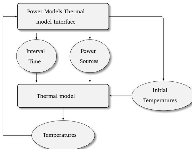
FIGURE 3.23: Thermal Simulation Flow
