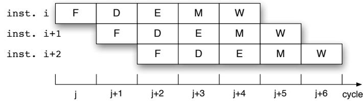
FIGURE 4.14: Pipeline of the ARM920T: Instruction is fetched in F. Instruction decode and operand register accesses are done in D. Execution is done in E. Load/store instructions do their memory accesses in M. Results are written back to registers in W.
