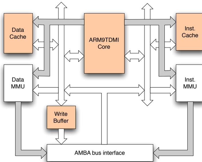
FIGURE 4.13: Simplified ARM920T architecture
