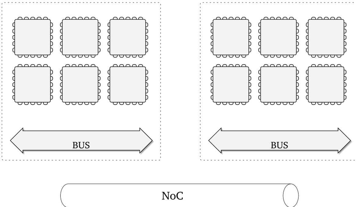
FIGURE 3.8: Double Hierarchy of communications in a modern many-core architecture
