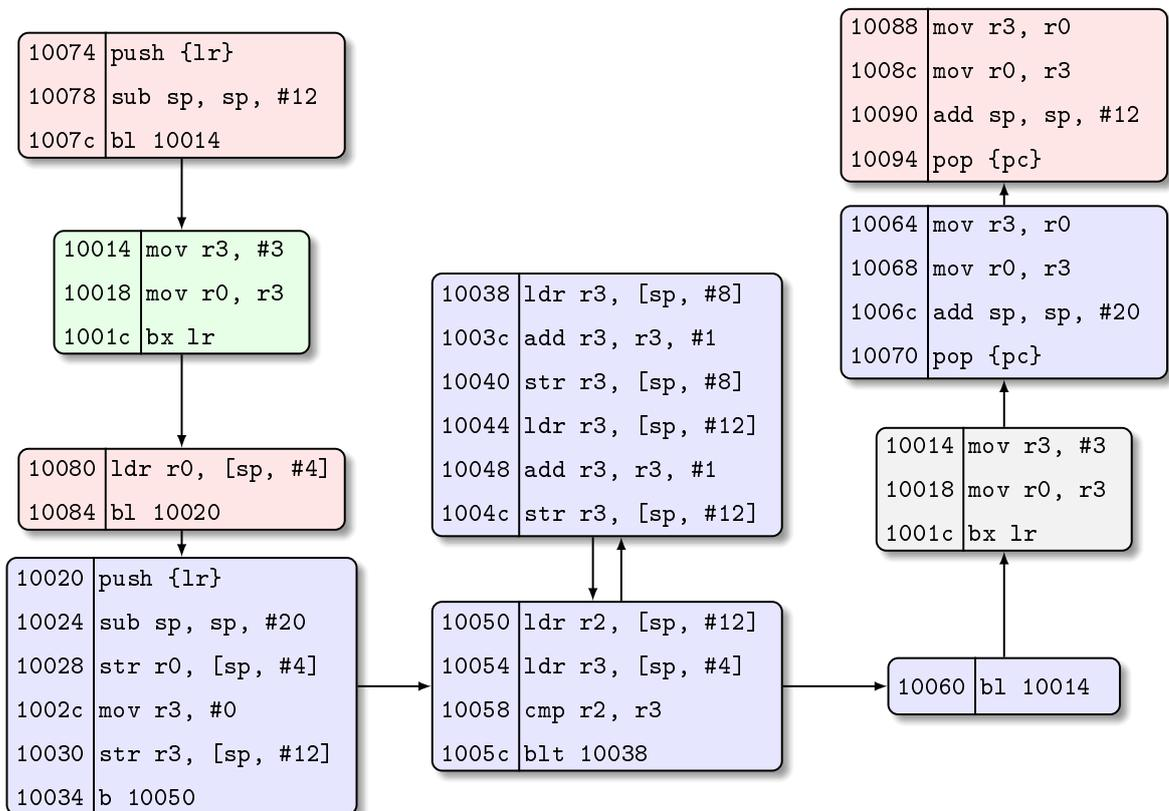
FIGURE 2.8: CFG of program in Figure 2.7
