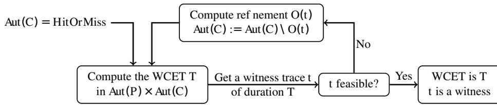
FIGURE 4.20: Trace Abstraction Refinement Algorithm for computing WCET
