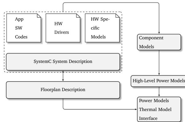
FIGURE 3.22: Simulation environment to estimate MPSoC temperatures
