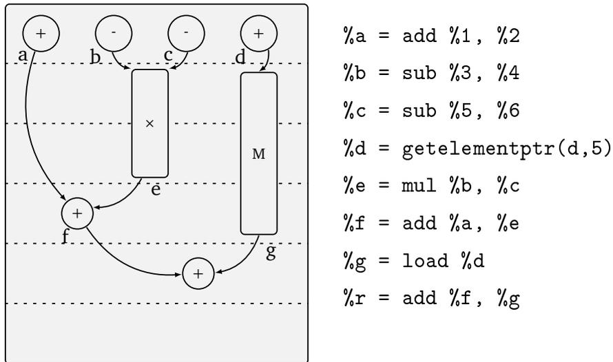
FIGURE 3.15: ASAP scheduling for eight simple operations, assuming that additions/subtractions take 1 cycle, multiplications take 2 cycles and memory accesses take 3 cycles.
