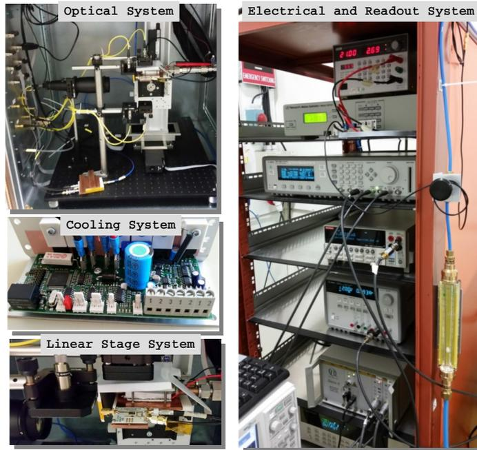
Figure 3.10: Pictures of the main systems of the TCT set-up at CERN: optical, cooling, linear stage, electrical and readout.
