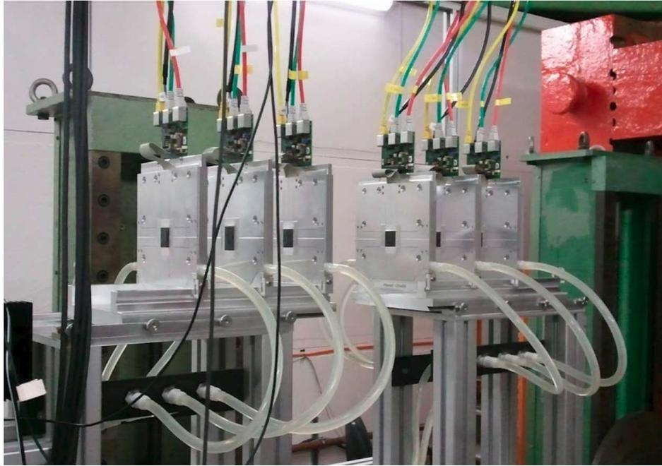
Figure 3.24: EUDET type beam telescope at DESY [50].
