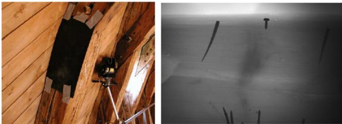
Figure 15 – Experimental Setup of X-ray Scanning (left) and Captured Image of a Wooden Beam with Metallic Elements Inside (right) (Riggio, et al., 2013).
