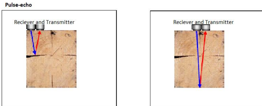
Figure 9 - Schematic of the Pulse-echo Method (Baron, 2009).
