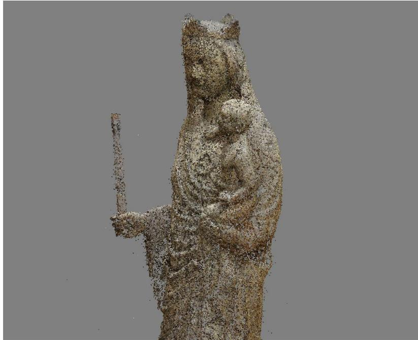
**Figure 1.1:** A 3D scanned point cloud of a Spanish Virgin wooden statue, kindly provided by the company 3DINTELLIGENCE.
