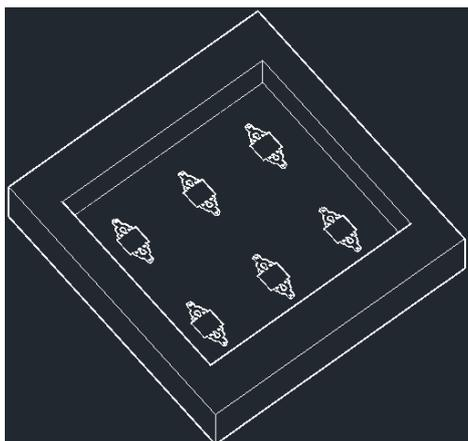
Figure 3: Final mold to create the chips. Here 6 chip designs were engraved to optimize the procedure and a resin wall was attached to ease the cutting process in the fabrication phase.
