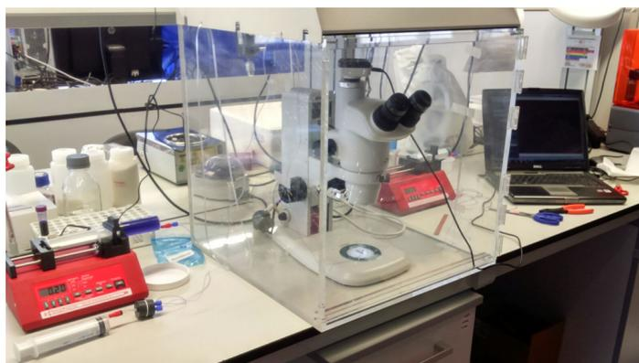
Figure 8: Setup for the microfluidics phase. On the side the computer in which the photos from the camera were recorded.
