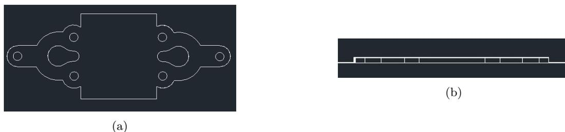
Figure 2: Design used for the chips that was obtained by the article from [9] and adapted to a 3.8mm x 9.81 mmx 0.24 mm format. (a) Top view of the chip, (b) side view of the chip.
