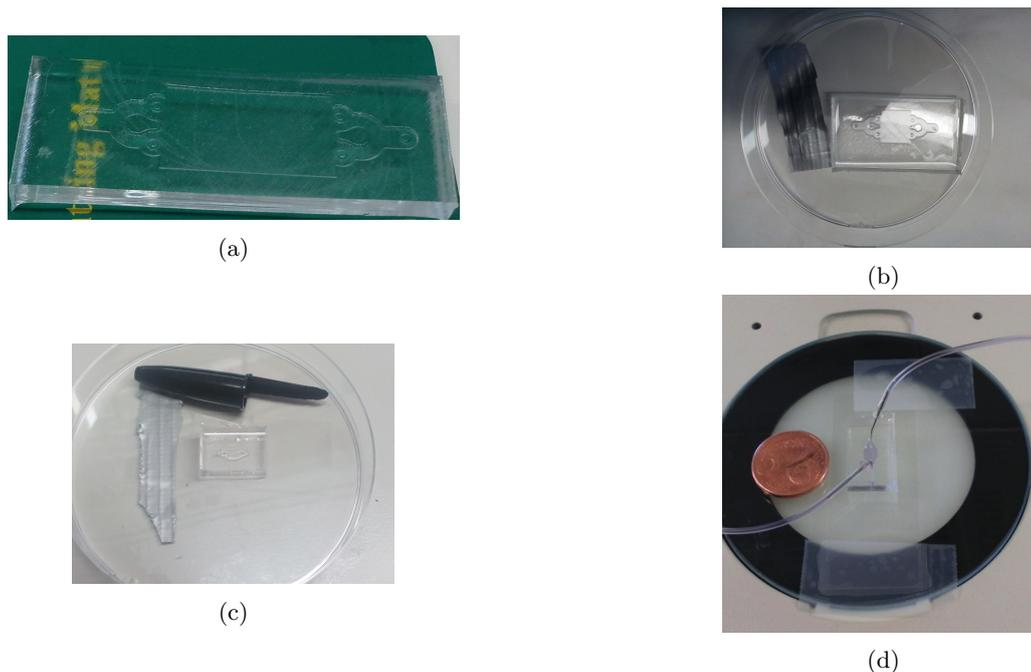
Figure 9: Images of the three different sizes of the chips. (a) The original size that was estimated from article [8], (b) The chip after reducing the chamber to half. Images (c) and (d) are the final chip that was used throughout the experiment.
