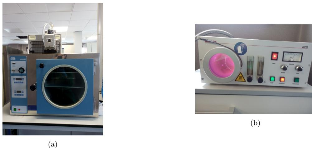
Figure 6: (a) The oven with vacuum used on the first day of the microfabrication process. (b) The O<sub>2</sub> generator used on the second day.
