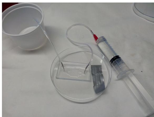
Figure 7: Image of the first quality check of a 33mm x 13mm x 0.24 mm PDMS chip.
