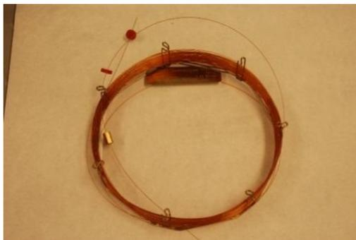
Figura 2.32. Columna HP-5 (30 m x 250  $\mu$ m x 0.25  $\mu$ m, Agilent Technologies).
