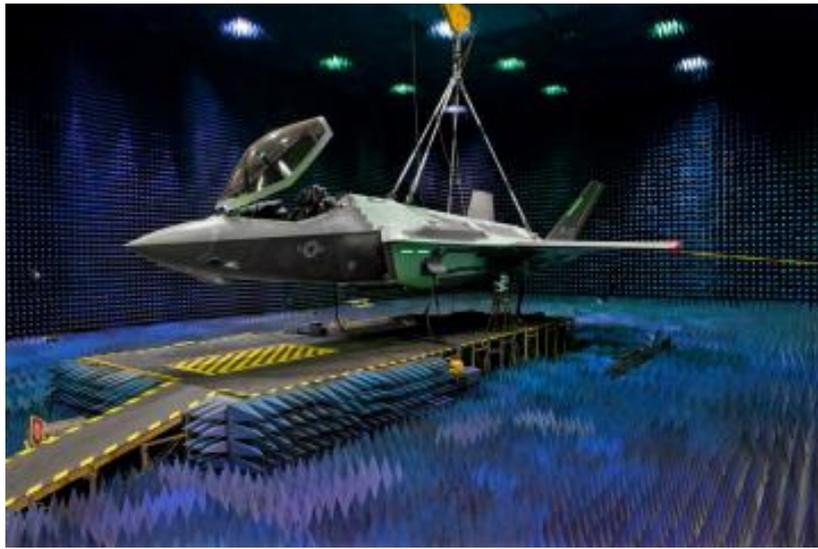
Figure 1.4: Photo of a radar cross section measurement in a anechoic chamber. Source: *Eletrical-GReece*
