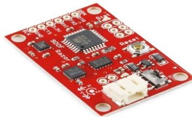
FIGURA 16 – RAZOR IMU 9DOF (<https://www.sparkfun.com/products/10736>)
