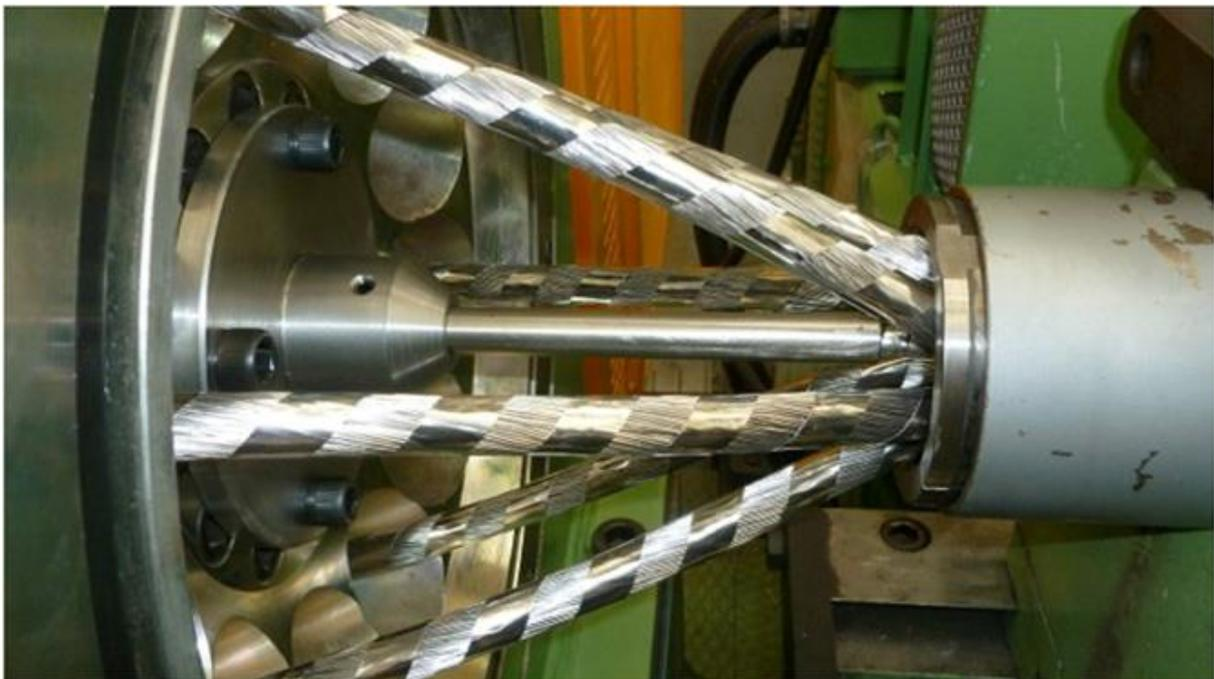
*Figure 3.4* final assembly for ITER TF cable [15].
