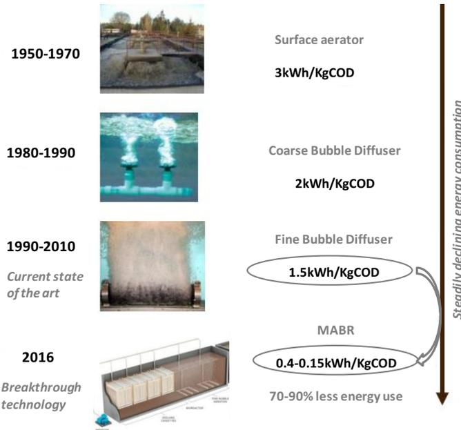
Figure 1-11 Evolution in wastewater aeration technology (adapted from www. emefcy.com).
