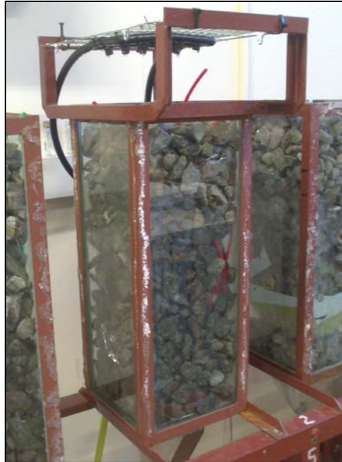
Fig. 1 Detail of the laboratory HFD model and the rainmaker.
