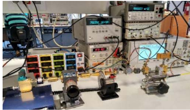
Fig. 7.32. Set-up to characterise the W-band radiometer in Dicke configuration.
