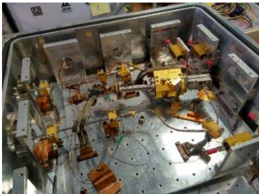
Fig. 6.25. FEM cryo- LNA placed in the cryostat just before a cooling cycle.
