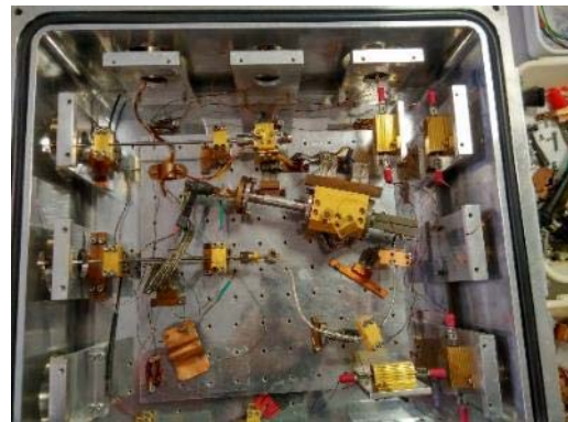
Fig. 6.25. FEM cryo- LNA placed in the cryostat just before a cooling cycle.
