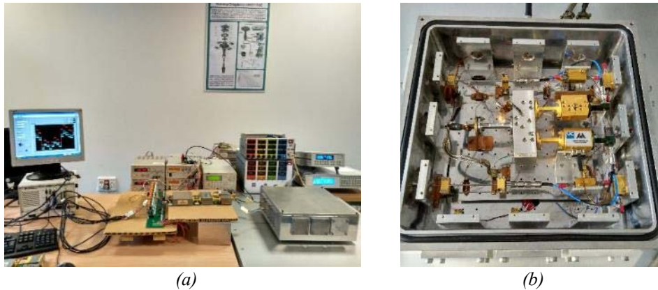
Fig. 6.32. FGI test-bench with the FEM cryo-LNA working at cryogenics. (a) General view of the BEM connected to the cryostat. The DAS is at the left-hand. (b) The two FEM LNA placed inside the cryostat and put together to the input load through and 3-dB coupler.
