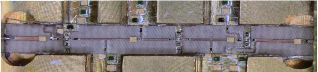
Fig. 3.32. Internal photo of the MIC LNA manufactured.
