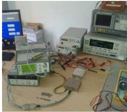
Fig. 6.18. Test set-up for DC to RF characterization for the Correlation and Detection Module of the FGI receiver.
