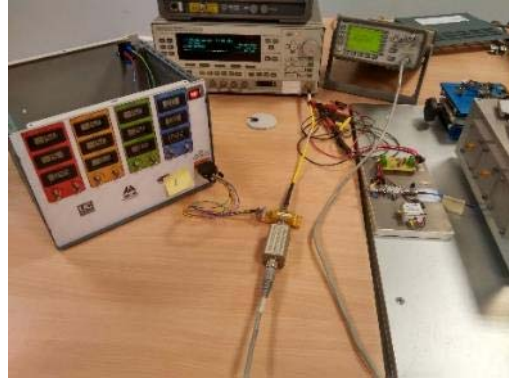
Fig. 3.39. P_{1dB} set-up for the MIC LNA at room temperature.
