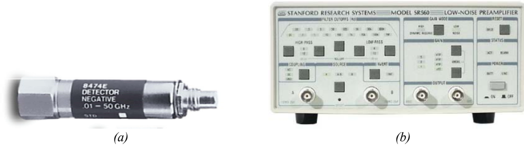
Fig. 7.25. Photos of the detector and video amplifier. (a) Detector from Hewlett Packard, reference HP8474E. (b) Low-noise pre-amplifier from Stanford Research Systems, reference SR560.
