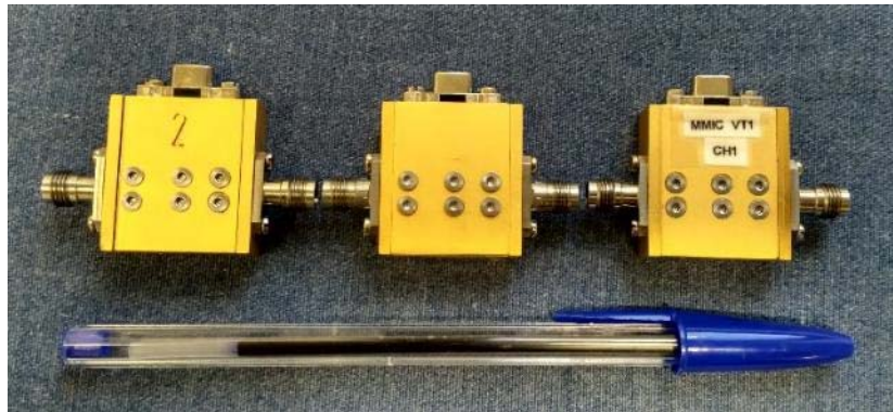
Fig. 2.28. Three chassis with the MMIC LNA assembled.
