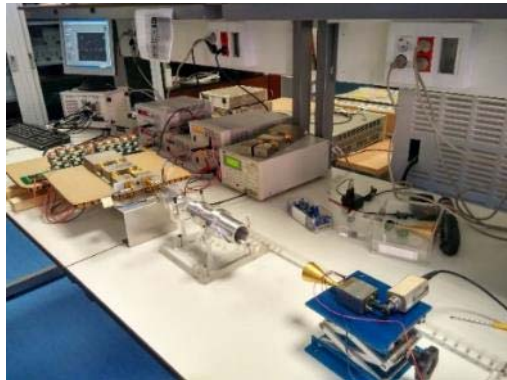
Fig. 6.21. Test-bench of the FGI receiver with the modular BEM.
