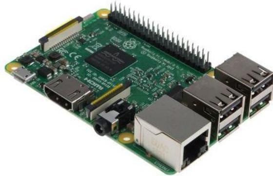
Figura 4.3. Raspberry Pi 3 Model B. Fuente: RS Components.
