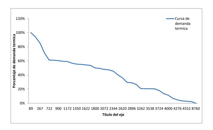
From this graphic is deduced that the value of the maximum rectangle is located within the 3694 hours with a percentage of 53%. This implies that the power needed to supply for each apartment is 1.556 KW. Therefore it is needed a machine of each type that can reach approximately 60 KW of thermal power.
