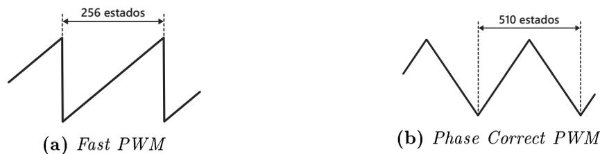
**Figura 4.16.** Modos PWM: *Fast* y *Phase Correct*
