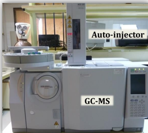
Figure 2.6. GC-MS Shimadzu QP2010 equipped with an auto-injector AOC-20i.
