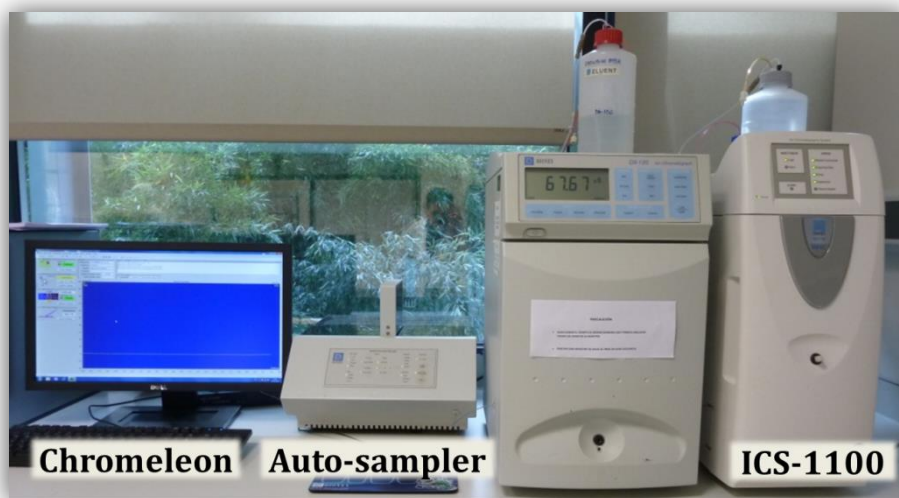
Figure 2.4. Ion chromatograph Dionex ICS-1100 equipped with a conductivity cell detector (ASR-ULTRA model).
