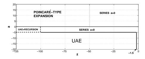
Figure 3: Methods for computation of the  $\gamma^*(a, z)$  function used in the final algorithm. UAE is the uniform asymptotic expansion of Section 2.3. The recursion relation is given in Eq. (2.12).
