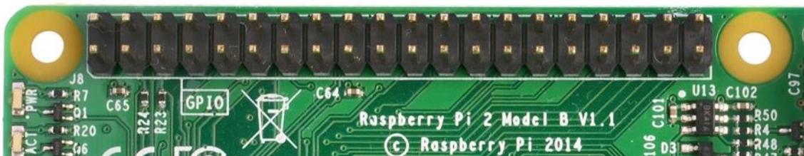
Figura 3.2. GPIO Raspberry Pi 3, General Purpose Input/Output
