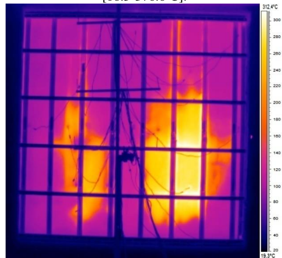
Fig. 15. Test 4: Temperature distribution at 165 min [19.3-312.4°C].
