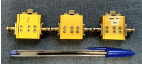
Fig. 11. Three chassis with the MMIC LNA assembled.
