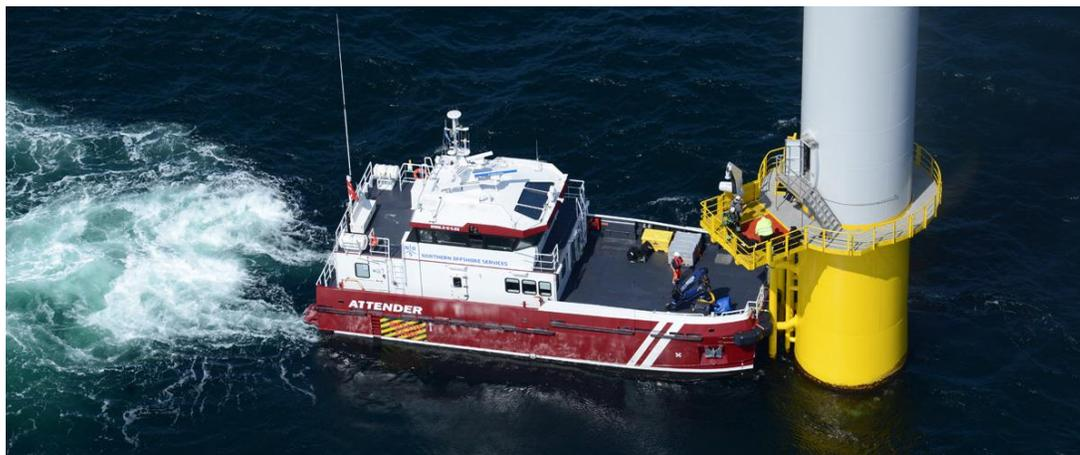
*Figure 14: Service vessel with fender, courtesy of Northern Offshore Services.*
