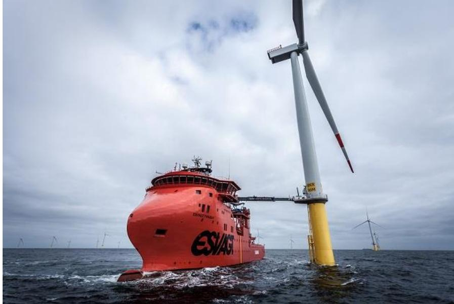
Figure 15: Service vessel with gangway, courtesy of Ampelmann.
