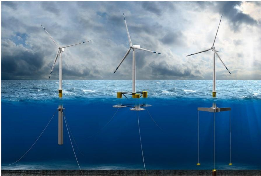
*Figure 8: Different concepts of floating platform for offshore wind applications (courtesy of DNV)*
