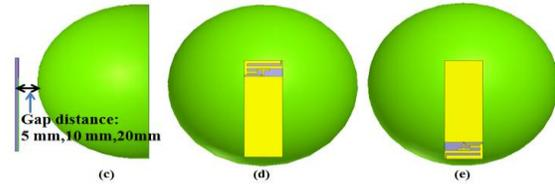
Fig. 2. Human head model. (a) Homogenous head model, (b) head model composed of seven layers, (c) gap distance, (d) antenna at the top position, (e) antenna at the bottom position
