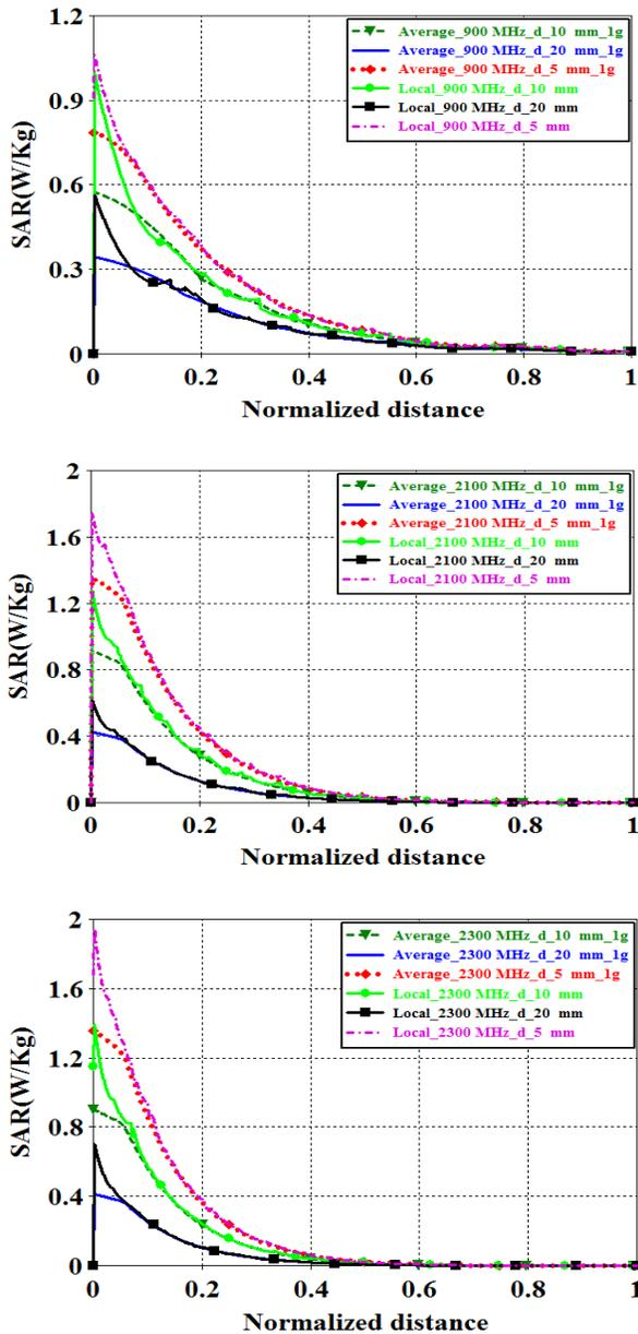
Fig.3. Local SAR and average SAR variation in 1-g head tissues for the homogenous head model, at different frequencies at various gap distances
