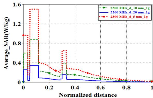
Fig.6. Averaged 1-g SAR distribution within the spherical seven layer head model, at various gap distances at different frequencies, the antenna is placed at the bottom position of the mobile phone
