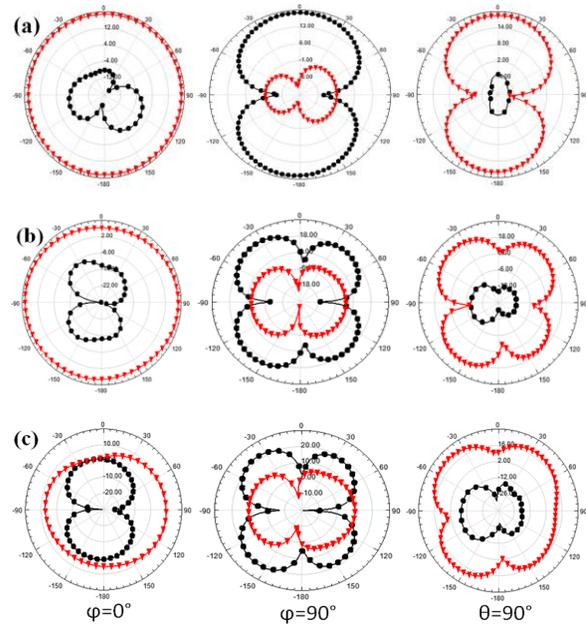
Fig. 8. Radiation patterns in 2D at (a) 900MHz, (b) 2.1GHz and (c) 2.3GHz for the proposed antenna (  $\blacktriangle$  dB(EPhi),  $\bullet$  dB(ETheta) )
