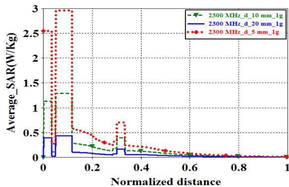
Fig.5. Averaged 1-g SAR distribution within the spherical seven layer head model, at various gap distances at different frequencies, the antenna is placed at the top position of the mobile phone
