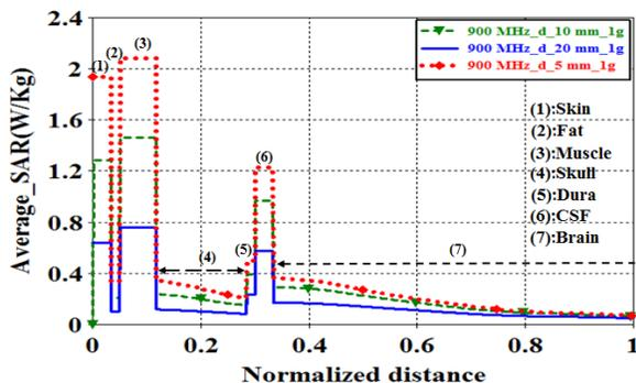
The comparison of the average 1-g SAR distribution inside the spherical seven layer human head model at various gap distances at different frequencies of 900 MHz, 2.1 GHz and 2.3 GHz are illustrated in Fig.6. In this case, the antenna is placed at the bottom of the mobile phone as shown in Fig.2(c). Results demonstrate that increasing the gap distance will lead to rapid decrease in the levels of the SAR.
