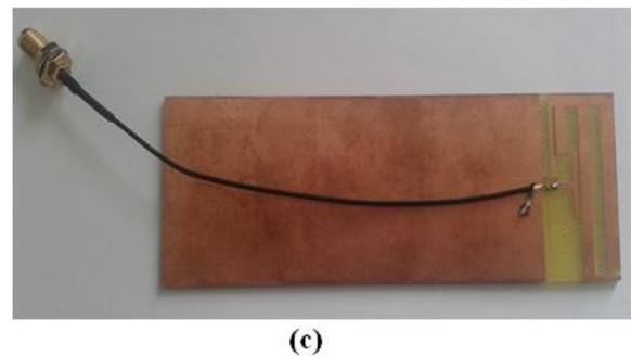
Fig.1. (a) Geometry of the antenna , (b) the metal pattern of the antenna and (c) photograph of the fabricated prototype of the proposed antenna
