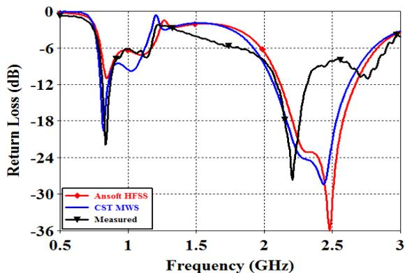
Fig. 7. Measured and simulated return losses by using CST MWS and HFSS for the proposed antenna
