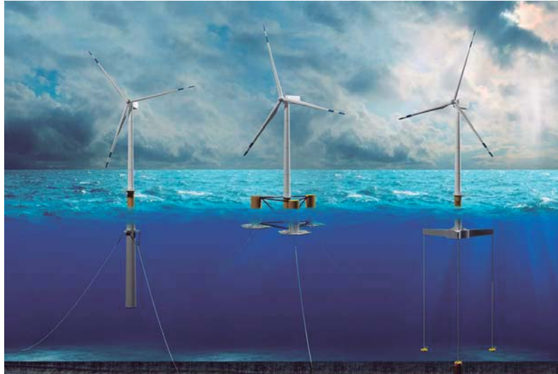
Figure 2.3: Offshore wind platforms concepts: (left) spar, (center) semisubmersible and (right) TLP
