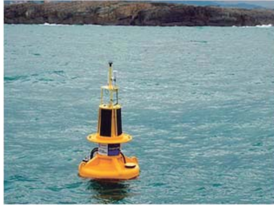
Figure 4.17: Red Vigía meteorological buoy (Source: www.redvigia.es ).
