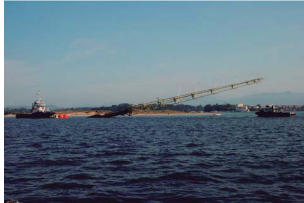
Figure 4.21: Idermar Meteo III floating met-mast during transport in 2011
