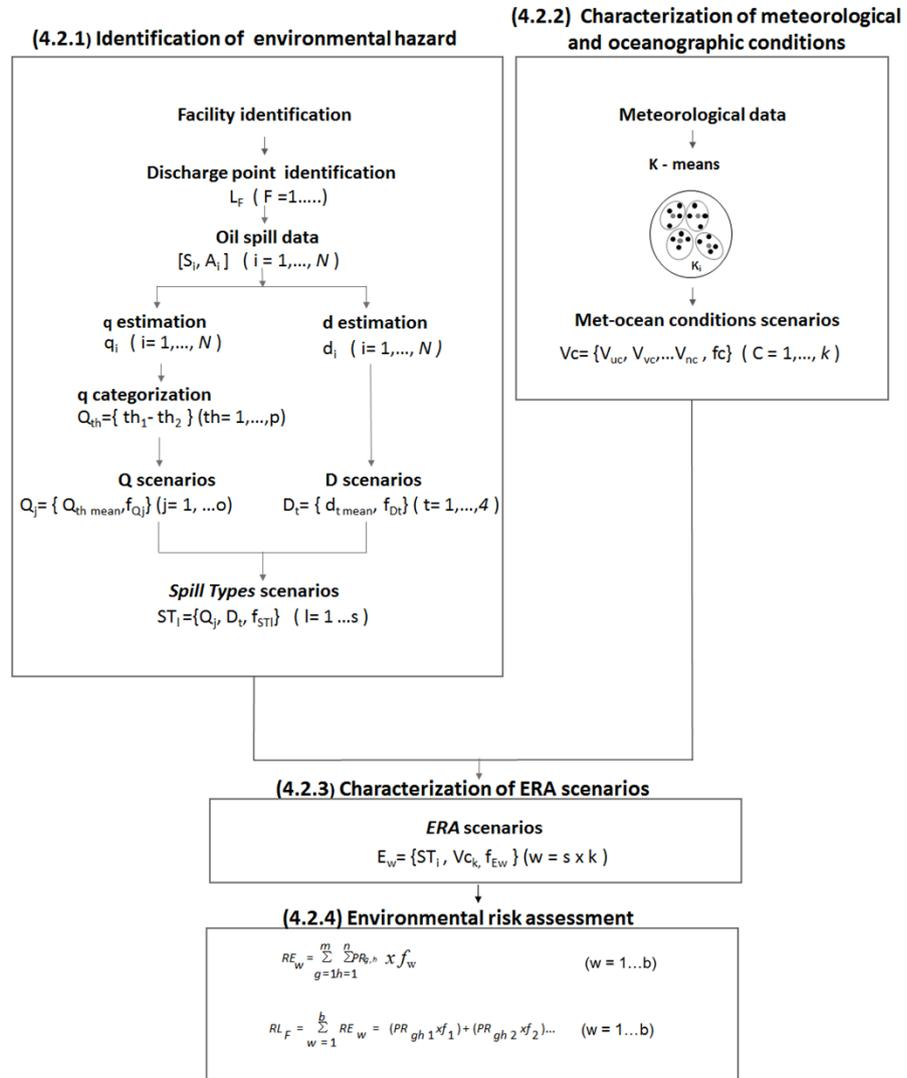
Figure 4.2 Schematic of the environmental risk analysis method for oil handling facilities in harbor areas.
