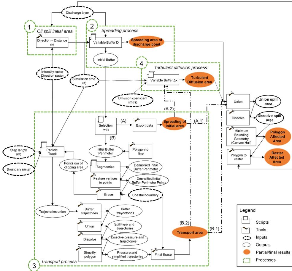
Figure 5.3 Graphic workflow representation of the SPILL Tool (1) Oil spill initial area process, (2) Spreading process, (3) Transport process, and (4) Turbulent diffusion process.
