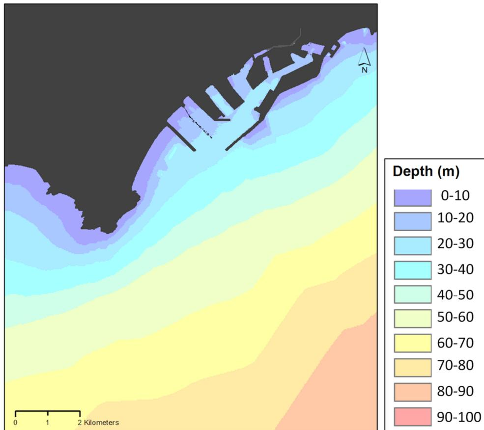
Figure 2.6 Representation of the bathymetry mesh grid at Tarragona harbor.
