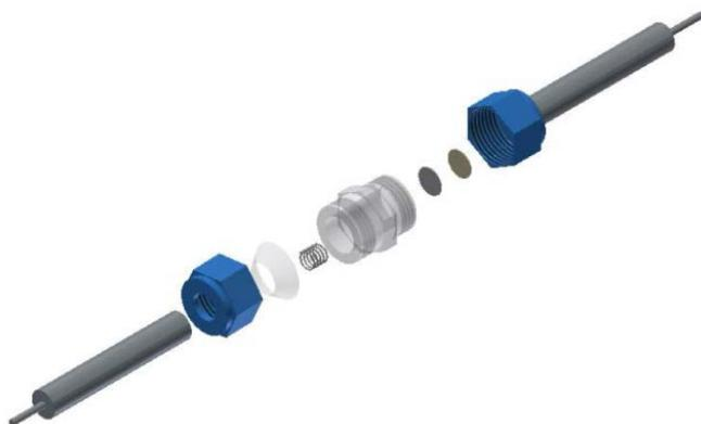
**Figure 2.2.** Homemade conductivity cell
