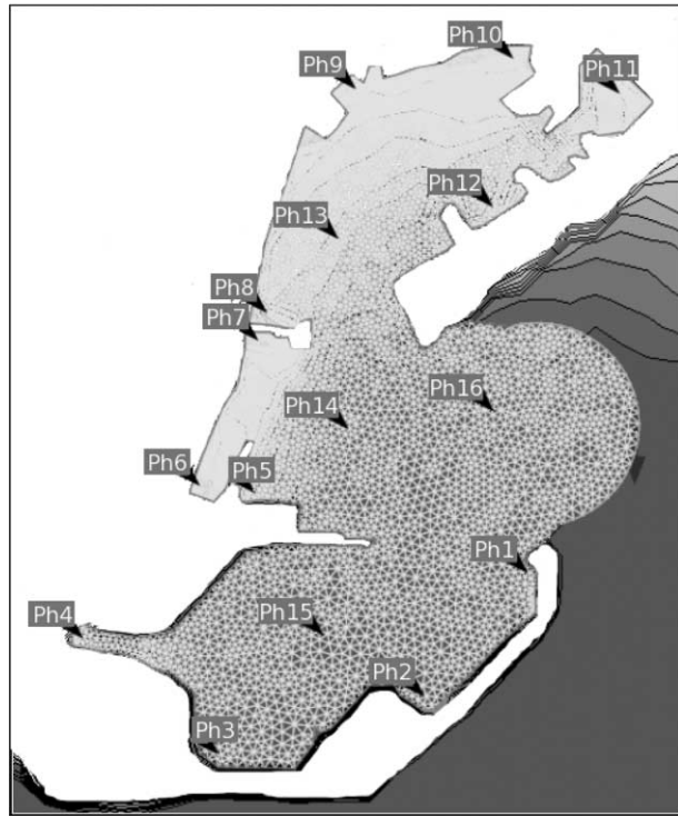
Figure 6. Domain used for Instituto de Hidráulica–mild slope simulations for the harbor of Palma, with location of the selected synthetic points. A color version of this figure is available online.
